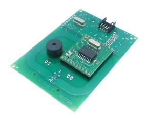
The PCB Multiplex Hitag is a modern and user-friendly RFID reader for easy integration into different applications.
