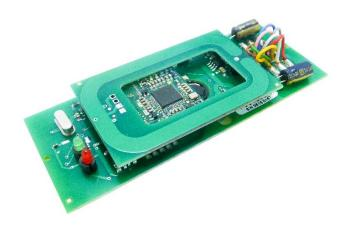
The RFID integration PCB Mini Multi ISO was developed for universal and easy integration into existing housings.
