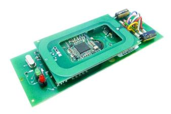
The RFID integration PCB Mini Mifare was developed for universal and easy integration into existing housings.
