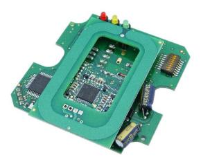
The RFID integration PCB MCR (Multi Card Reader) Multi ISO was developed for universal and easy integration into existing housings.
