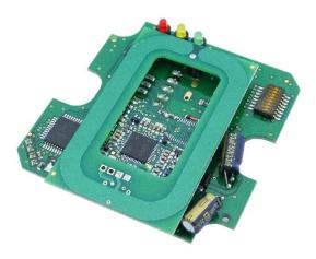
The RFID integration PCB MCR (Multi Card Reader) Mifare was developed for universal and easy integration into existing housings.
