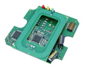
The RFID integration PCB MCR (Multi Card Reader) LEGIC was developed for universal and easy integration into existing housings.
